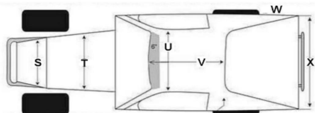
**SAIL PANELS:** Must not be wider than the body and must attach to the quarters in a single stock appearing plane that angles inward to the roof. No fins or lips on sail panels, body or nose
